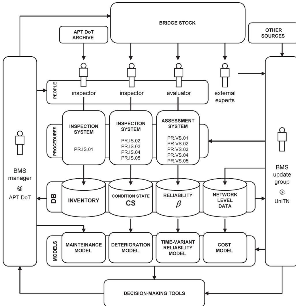
Figure 2. Layout of the APT-BMS showing its main components and information flows.
