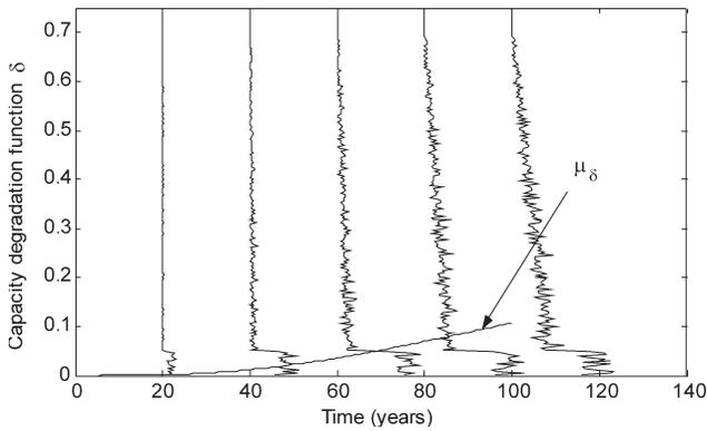
Figure 7. Capacity degradation function for a limit state associated with Element #12 (concrete deck).
