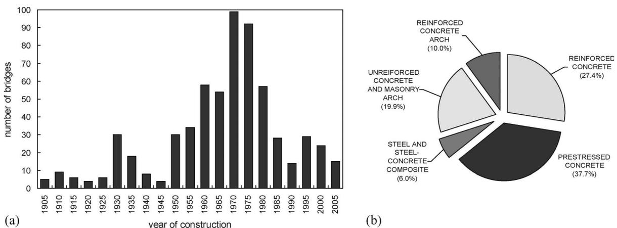
Figure 1. Bridge age distribution (a) and typological distribution (b) in APT.
