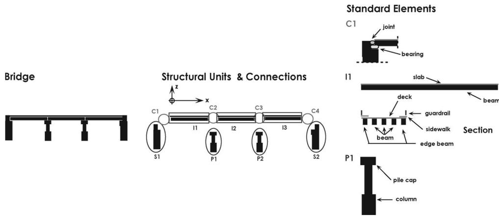
Figure 4. Example of bridge representation and break down into Structural Units and CoRe Standard Elements (AASHTO 1997), as implemented in the APT-BMS.
