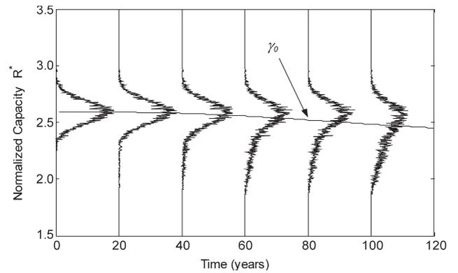
Figure 8. Time variant normalized capacity PDF for a limit state associated with Element #12 (concrete deck).
